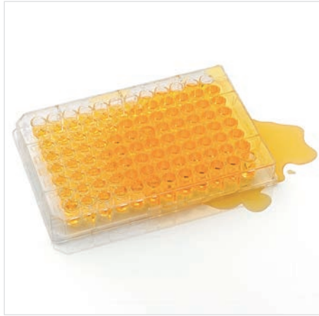
Spilling of plate caused by clogged needles
