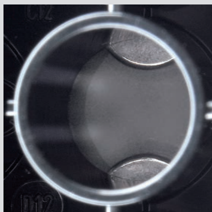
Optimized bead recovery using two magnets per well
