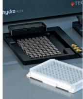
Patent pending plate carrier for magnetic bead separation (MBS) for washing bead-based assays
