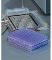
8- or 16-way manifold for ELISAs and cell-based assays, allowing simultaneous washing of 8 or 16 wells
